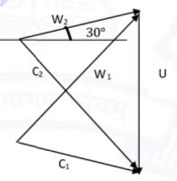
The blade speed (U) at the mean radius of the rotor is \_\_\_\_\_ m/s (round off to two decimal places).
